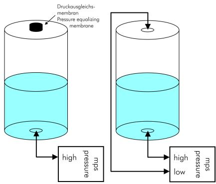
has to be installed into a top port of the reservoir (valid for all sensor types). If the port "low" is used, the hose connecting this port to the top of the reservoir has to be filled with air. Otherwise, the sensor will produce erratic readings and the actual fill level may differ significantly from sensor reading! Aqua Computer therefore
