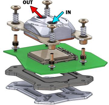
ing one of the knurled head screws (only one or two revolutions). Alternately fasten each screw a fraction of a revolution until all four screws are fully fastened.
