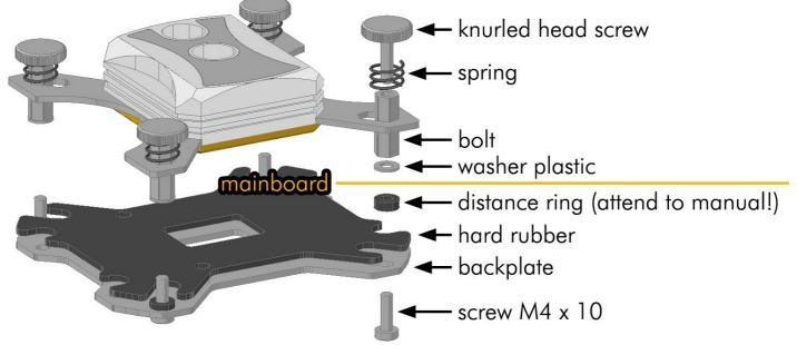
Orientate the bolts to suit the apertures in the cuplex kryos. To do so, you might need to loosen the screws a bit and then refasten the screws. Slide the cuplex kryos onto the bolts and carefully lower it onto the thermal grease covered CPU. Apply one of the four supplied springs to each bolt and secure each spring using one of the knurled head screws (only one or two revolutions). Alternately fasten each screw a fraction of a revolution until all four screws are fully fastened.
