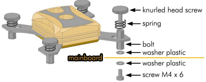
Orientate the bolts to suit the apertures in the cuplex kryos. To do so, you might need to loosen the screws a bit and then refasten the screws. Slide the cuplex kryos onto the bolts and carefully lower it onto the thermal grease covered CPU. Apply one of the four supplied springs to each bolt and secure each spring using one of the knurled head screws (only one or two revolutions). Alternately fasten each screw a fraction of a revolution until all four screws are fully fastened.
