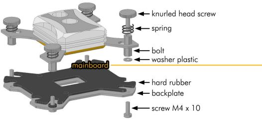
the knurled head screws (only one or two revolutions). Alternately fasten each screw a fraction of a revolution until all four screws are fully fastened.
