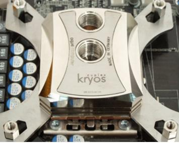
The internal design of the cuplex kryos is not symmetrical, most current CPUs are also not symmetrical (below the heat spreader cap). Therefore the cuplex kryos should be aligned to the CPU socket as shown in the figure.
