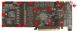
lift the air cooling unit off the graphics card while disconnecting the fan connector.
