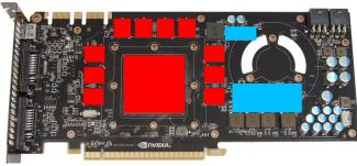
Apply a thin layer of thermal compound to the GPU and the RAM modules. These components are marked red in the figure. The thermal compound must not be electrically conductive! Cut fitting pieces from the thermally conductive pad supplied with the aquagraFX and place them on top of the voltage regulators as indicated by blue rectangles.
