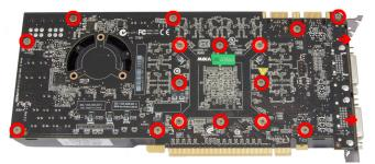
in the figure. Use extreme caution not to damage any of the highly sensitive components of the graphics card! Disconnect the fan connector while lifting the air cooling unit off the graphics card.
