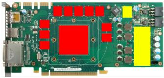
ting pieces from the thermally conductive pad supplied with the aquagraFX and place them on top of the voltage regulators as indicated by yellow rectangles.
