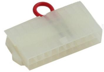
Please note: Some high-power PSUs will not be able to power the aquaduct without further electrical load due to power regulation problems. In this case, use a second (complete) PC or a separately sold PSU for single component for the filling process. Alternatively, connect further load like hard disk drives and optical drives to the PSU.
