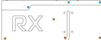
Blue marking: Three screws M2,5 x 8 mm, countersunk head.
