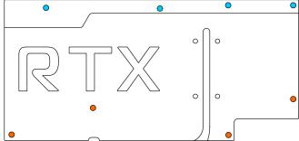
Blue marking: Four screws M2,5 x 8 mm, countersunk head.
