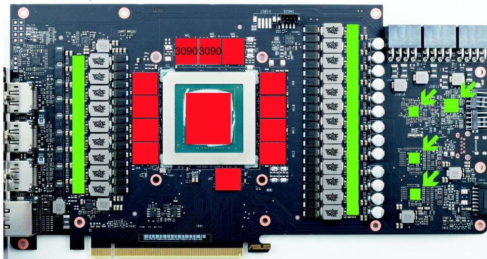
Apply a thin layer of thermal compound to the GPU and the RAM modules (ten RAM modules for 3080, twelve for 3090). These components are marked red in the figure. Place the pre-cut thermally conductive pads with the kryographics on top of the components as indicated by green rectangles.
