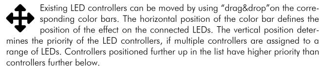
The length of the bar (corresponding to the number of LEDs assigned) can be changed by moving the right/left edge of the color bar.
