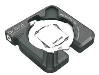
Fasten the screw until the heat spreader comes loose.
