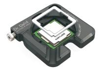
After cleaning, apply new thermal grease onto the die.
