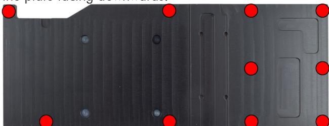
Place one black plastic spacer supplied with the back plate into each of the 10 recesses of the back plate marked red in the figure.
